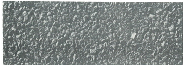
Excellent surface texture of lightweight aggregate coverstone after five million vehicle applications-photograph taken in the wheel path
