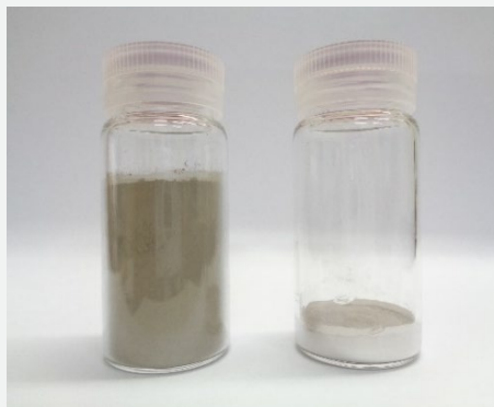
Fig. Silver powder (10g) (←) Dendritic silver powder (→) Conventional silver powder
